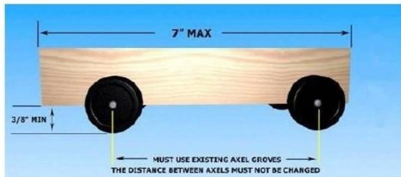
**Figure 2: Length, Height, Wheelbase, & Clearance Requirements**
